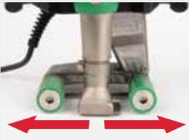
**Customized:** Reversible drive allows for welding in either direction
