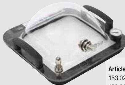
For testing T-joints
