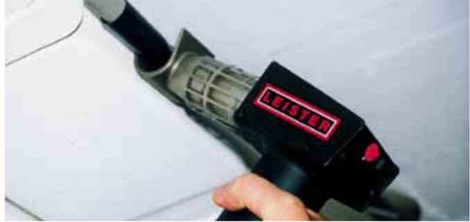
Shrinking cable connections with the GHIBLI.
