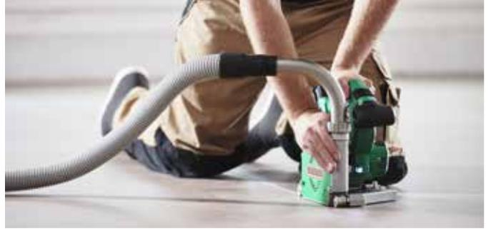
The vacuum cleaner adapter allows to connect the tool to a vacuum cleaner. Highest suction performance is guaranteed.
