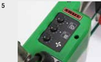
**5** **UNIROOF ST for purists: Closed-loop controlled drive motor with open-loop technology** for the control of temperature and air blower. Simple control (regulation) with potentiometer/rotary knobs.
