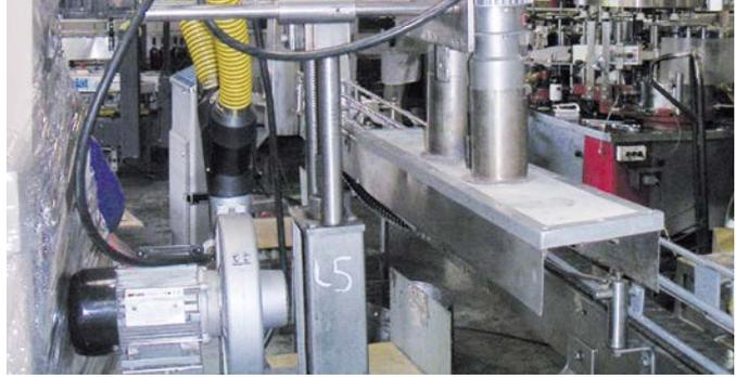
Two LE 10 000 HT air heaters and an ASO blower in combination with a shrink tunnel.
