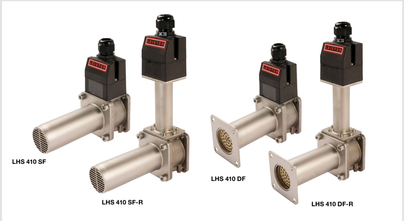
The housing connection on the LHS 410 is located outside the air flow, allowing the air to flow through the air heater unhindered and with hardly any loss in pressure. In addition, the housing connection of the LHS 410 SF-R and DF-R is protected against overheating, making it possible to work with air inlet temperatures up to 662°F.
