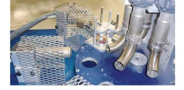
High-end air heaters on an indexing table for producing light bulbs.
