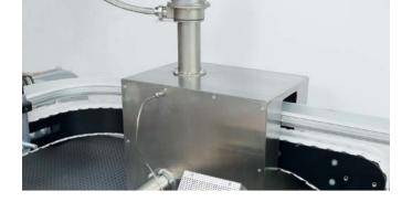
Energy efficient hot-air recycling with LE 5000 DF-R air heater on a shrink tunnel.
