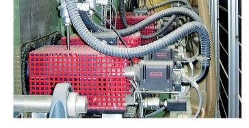
LHS air heaters in a production line for drying insulating material.
