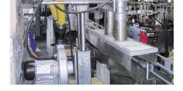
Two LE 10 000 HT air heaters and an ASO blower in combination with a shrink tunnel.
