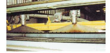
Two air heaters and two blowers used to dry impregnated Eternit piping. Two wide slot nozzles ensure the air is evenly distributed.
