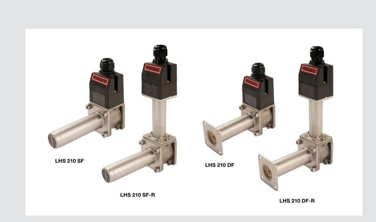
The housing connection on the LHS 210 is located outside the air flow, allowing the air to flow through the air heater unhindered and with hardly any loss in pressure. In addition, the housing connection of the LHS 210 SF-R and DF-R is protected against overheating, making it possible to work with air inlet temperatures up to 662°F.
