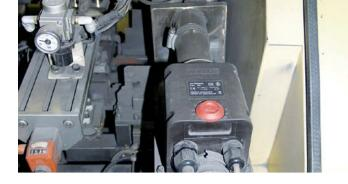
Deflashing foil sleeves from charcoal filter elements
