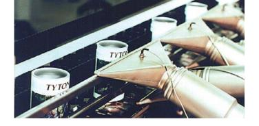
Utilizing precisely controlled hot air to shrink PE sleeves on cans.
