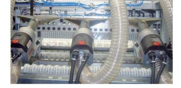
Three LHS 61S air heaters with wide slot nozzles in a wrapping line.
