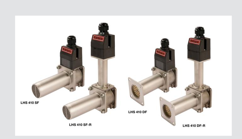
The housing connection on the LHS 410 is located outside the air flow, allowing the air to flow through the air heater unhindered and with hardly any loss in pressure. In addition, the housing connection of the LHS 410 SF-R and DF-R is protected against overheating, making it possible to work with air inlet temperatures up to 662°F.
