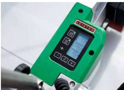
Regulated welding parameters
