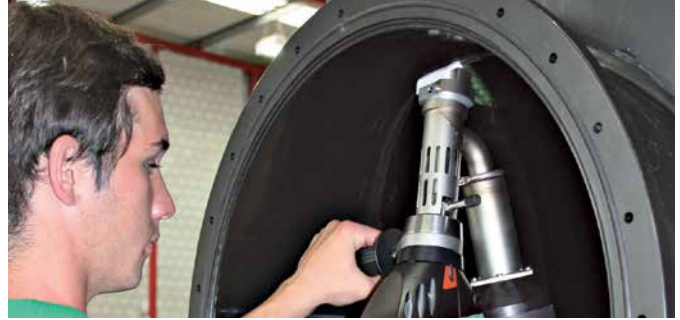
Even inside radiuses are easy to weld
