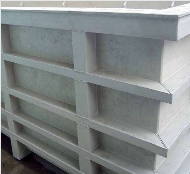
Electroplating tank, Turkey. Material: PP
