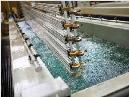
Galvanic bath made of polypropylene © Collini collini.eu
