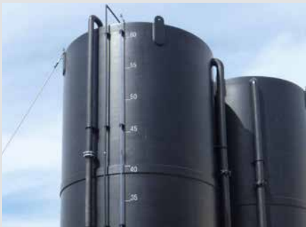
Storage tanks made of polyethylene
