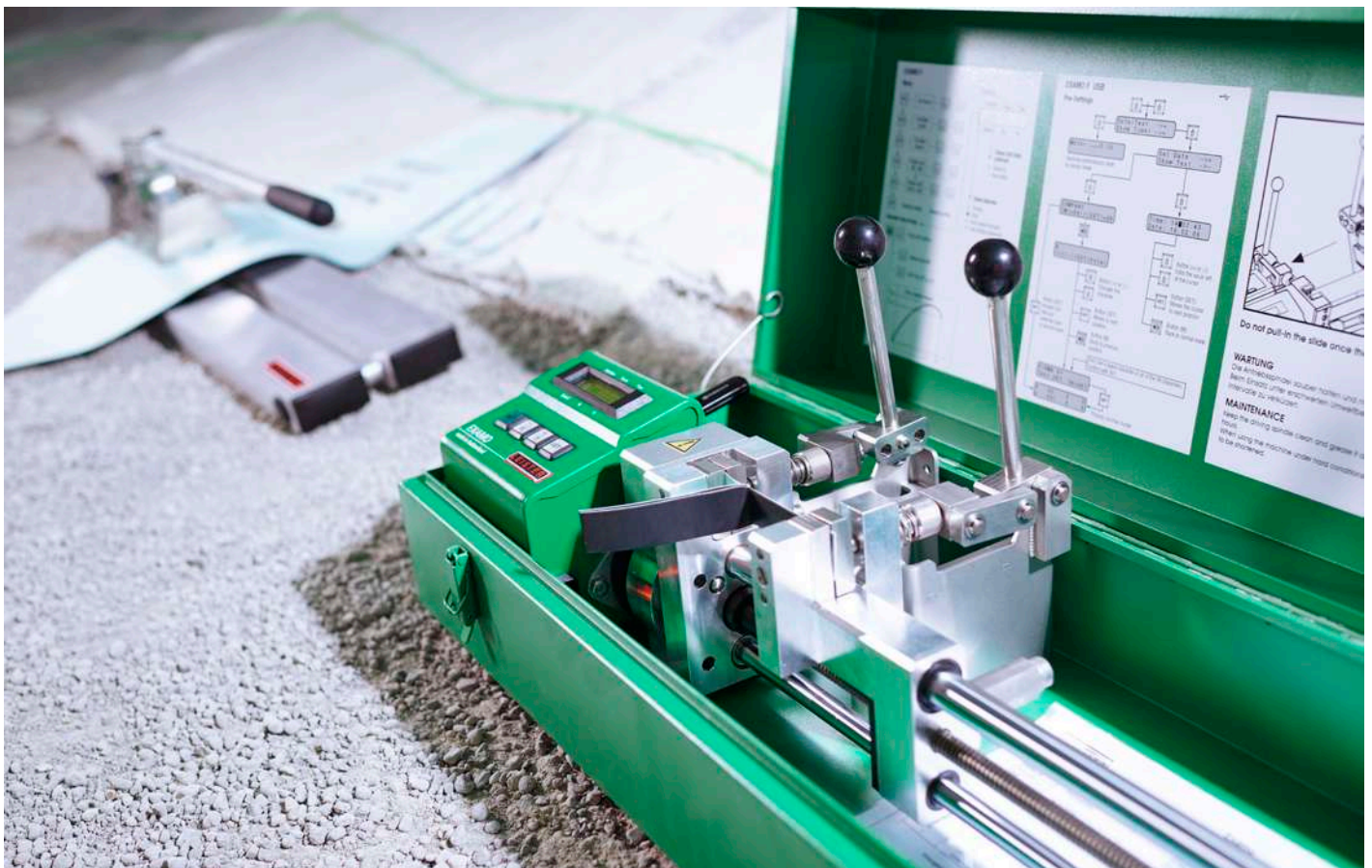
Strength testing of an overlap weld seam with the EXAMO 300F USB from Leister
